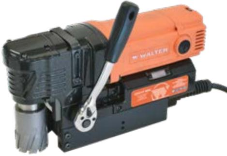
Measuring in at only 7-inches tall, the ICECUT MINI™ is the ultimate compact, low-profile magnetic drilling unit for making holes in tight spaces from H-beams to truck frames, and other applications where space may be limited. This unit has a powerful electromagnet for safety while drilling and **has a 2" x 2" drilling capacity**, making it the most versatile unit in its class.
