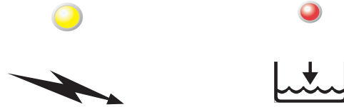
Indicator for wand tip power ON
